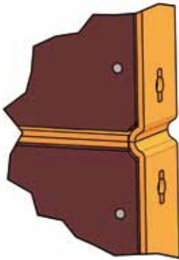
Detail of Modular formwork elements (element joint)
