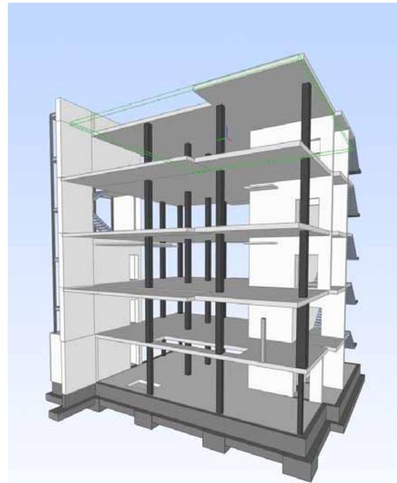
*The fully automatic PPL 11.0 formwork software reads in the BIM data via the integrated IFC interface and generates the ideal formwork complete planning from the data.*
