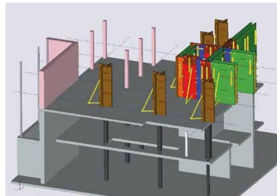
*The formwork planning can be displayed, issued, calculated and kept track of section by section and in phases. In this way, work scheduling and construction management always have an overview of the construction project.*
