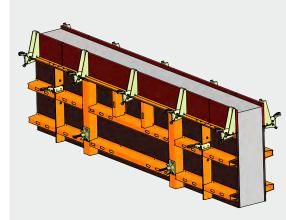
If small panel widths (used horizontally) are not sufficiently available, extension brackets can be used for height extensions.
