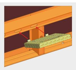
For assembly, the step is at a slight angle to allow the mounting brackets to be inserted into the elongated holes on the panel cross sections.
