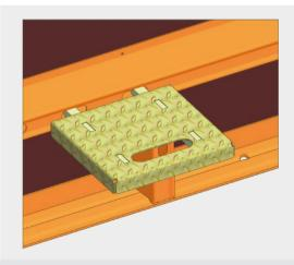
The step is then folded down to provide a safe working area.
