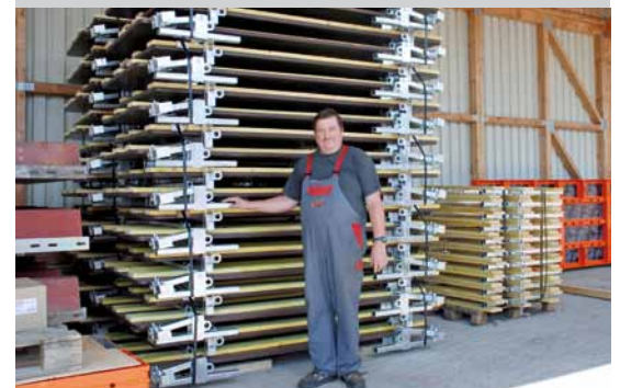
Concreting platforms can be folded for transport or storage to save space.
