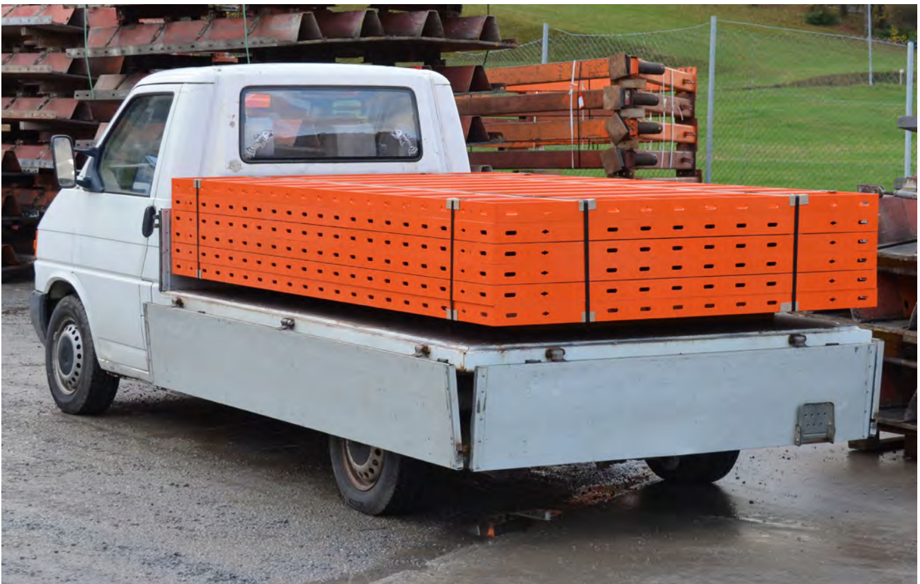
Due to the low weight and the ideal product dimensions, up to 6 large-size panels (1.116 kg) can be transported with a flatbed truck.
