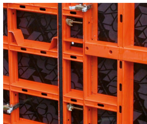
Fillers up to 12 cm can also be fixed between two panels using a locking screw.
