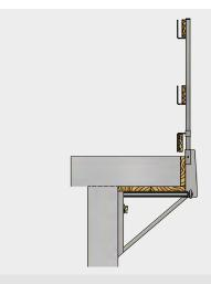
The stop can be moved by 50 cm for concreting brackets.
